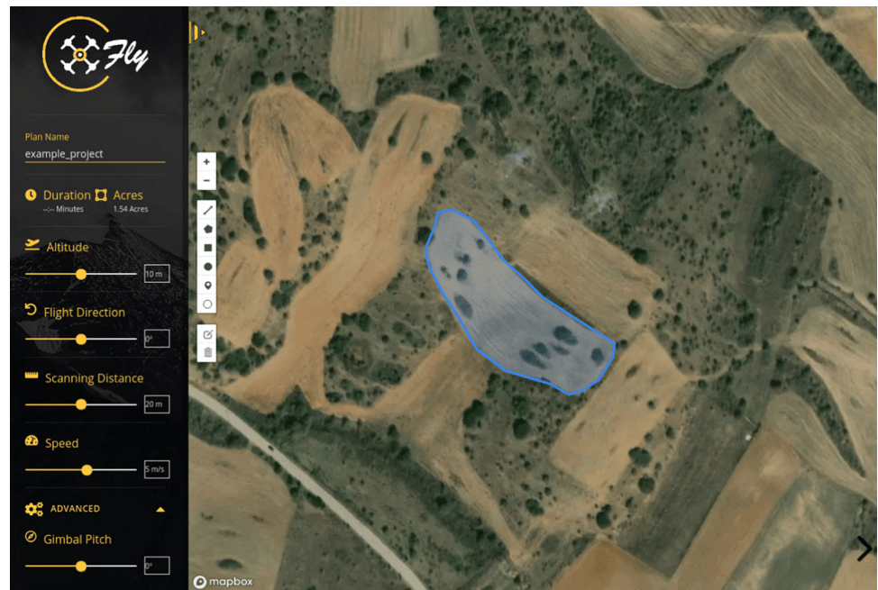
Fig. 12 CoFly GUI, showing the available flight settings menu bar on the left, and the map with the polygon drawn by the user
